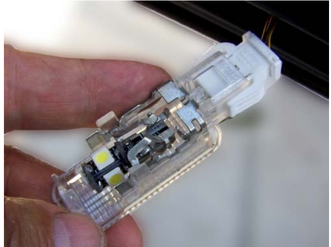
The puddle lamps also take a 5-chip LED.
